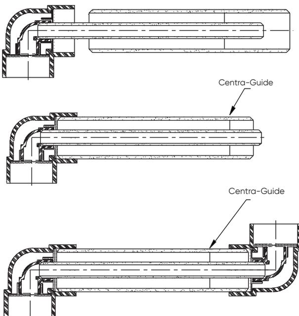
1. Determine proper carrier and containment pipe lengths to achieve desired center-to-center dimension. Cut to size and prep ends.
