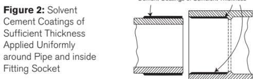
**Figure 2:** Solvent Cement Coatings of Sufficient Thickness Applied Uniformly around Pipe and inside Fitting Socket
