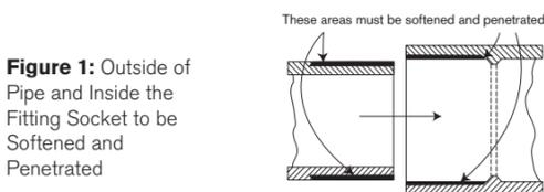
**Figure 1:** Outside of Pipe and Inside the Fitting Socket to be Softened and Penetrated
