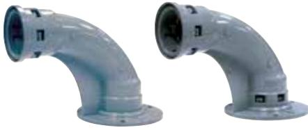
Both styles of stub down fittings are designed for direct connection to ENT on the horizontal by means of our unique six locking tab for concrete encasement Kwikon connection. The flanged base of the threaded 90° stub down offers contractors a NPSC threaded hub connection on the vertical – at the exit point of the slab, allowing for the direct transition to other raceway products.
